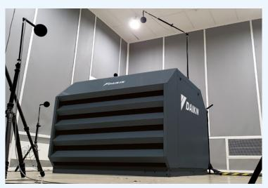
Sound power level measurement in acoustic chamber
