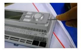
Be careful to avoid damages to the plastic cover. The new battery shall be placed in the proper battery holder which is highlighted in the following picture, respecting the polarities indicated into the holder itself.
