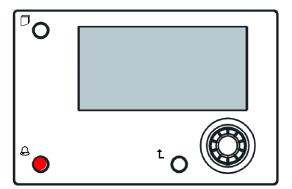
The Remote can be ordered with the unit and shipped loose as a field installed option. It can also be ordered anytime after chiller shipment and mounted and wired on the job as explained on the following page. The remote panel is powered from the unit and no additional power supply is required.
