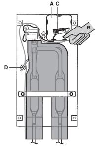
4 Use a small screwdriver and follow indicated instructions for connecting cable wires into the terminal connector according to the wiring diagram.
